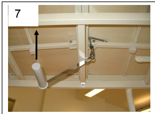
Lift the handle upwards a little at the same time as placing the hook between the white strut and the wooden board.
