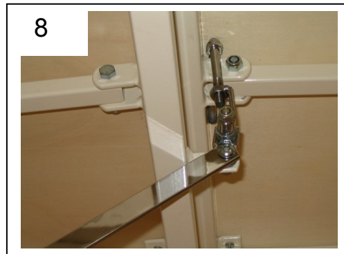
Place the hook between the crossbar and the bolt. When done correctly it should look like picture 8 and 9
