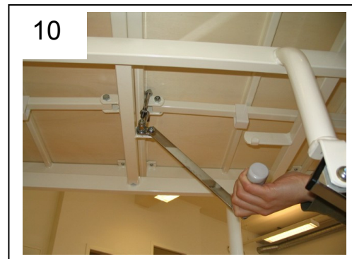
Lift the handle upwards and hook it in position, see picture 11 and 12. If it is almost impossible to lift the handle upwards or if the couch doesn't seem to be fastened properly; adjust this by unscrewing or screwing the hook
